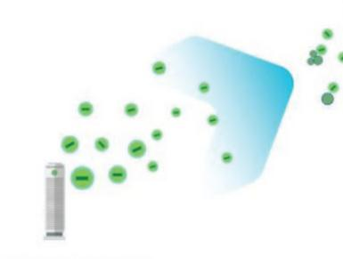
An air ionizer electrically charges the surrounding air or oxygen ions to produce charged particles negatively charged oxygen ions(O2-)
